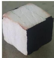
Fig. 2.4 Wood coated with conductive ink
