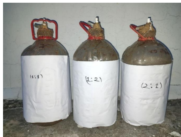
Fig. 2 Treatments mixed Napier grass and banana peel in 1:1, 1:2, and 2:1 ratios (by mass), with a fixed amount of cow dung.
