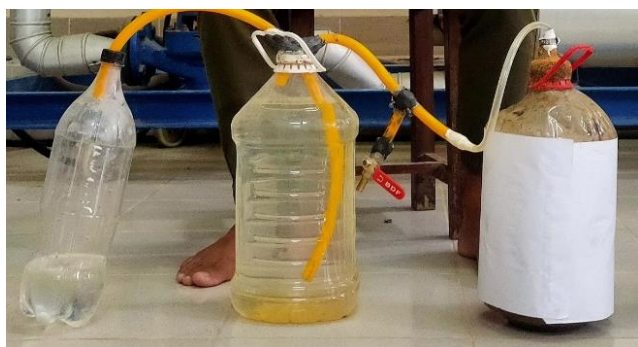
Fig. 3 Digester construction and setup.
