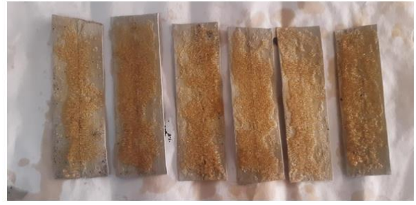
Fig. 4: PDMS treated aluminium sheet
