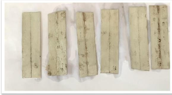
Fig. 3: Sulfuric acid treated aluminum sheet
