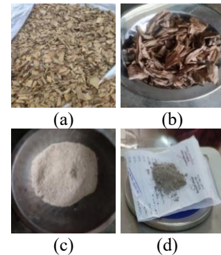
Fig.2: (a) Sundried water hyacinth after 15 days; (b) Oven dried water hyacinth after 3 days; (c) Water hyacinth ash after burning at furnace; (d) Water hyacinth ash after sieve.
