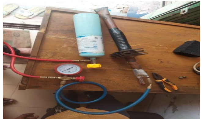
Fig.1 Working fluid enters the heat pipe
