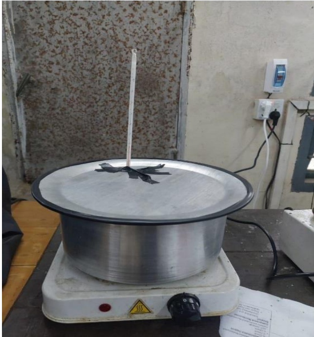
Fig.2 Experimental setup of natural cooling without a heat pipe
