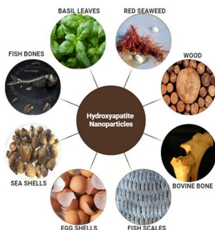
Fig.1 Schematic Diagram of HAp Sources.
