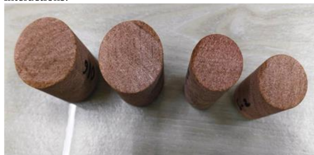
Fig. 4. Core samples after acid treatment
