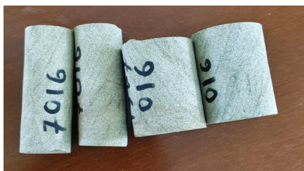
Fig. 3. Prepared core samples before acid treatment
