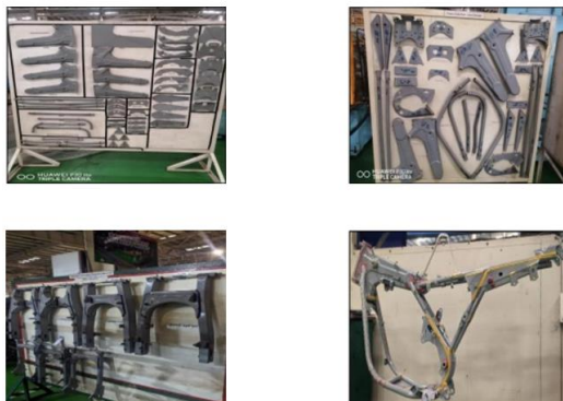
Fig. 10: Arrangement of component using 5S
