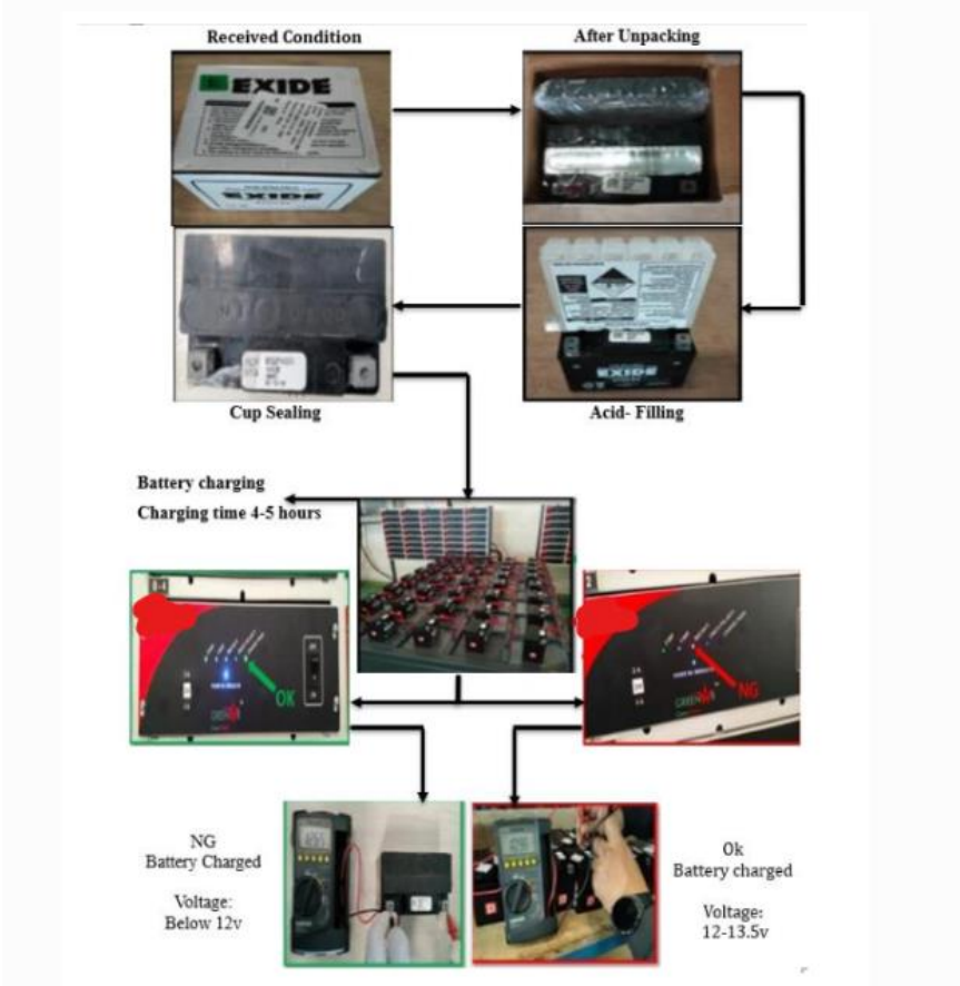
Figure 8: Standard Battery Charging Procedure & Monitoring
