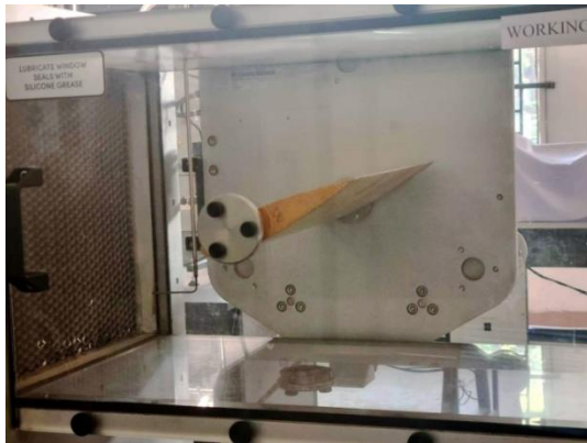
Fig.7: Experimentation of dimpled airfoil using wind tunnel
