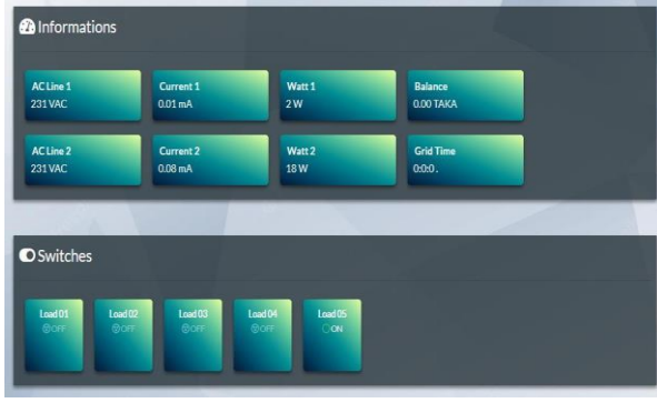
Fig. 5 IoT Web dashboard for load monitoring.
