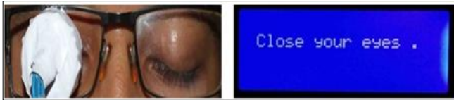
Fig. 7: Instruction is shown on LCD to take value of closed eyes
