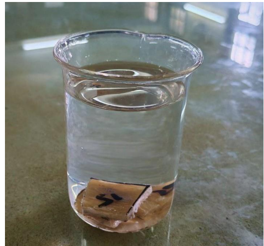
Fig 4: Water Absorption Test.
