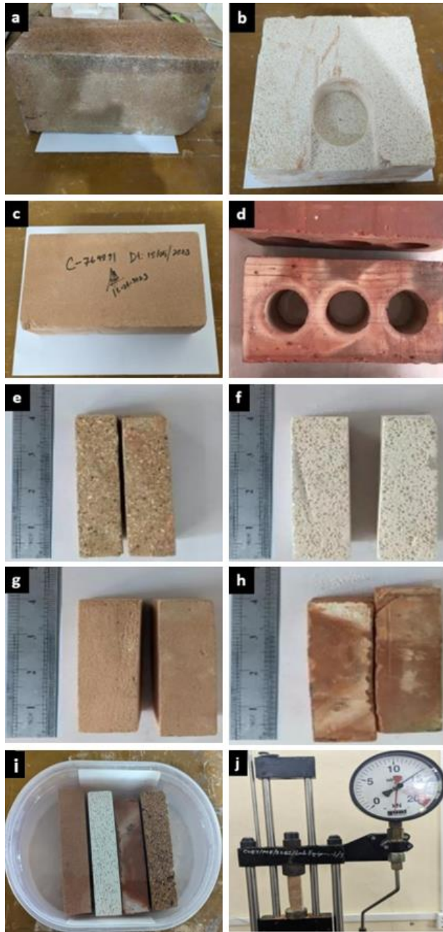
Fig. 1: Images of a) furnace brick type-1 (FB1), b) furnace brick type-2 (FB2), c) furnace brick type-3 (FB3), d) conventional brick (CB). Test specimens of e) FB1, f) FB2, g) FB3, h) CB. i) brick specimens soaking in water. j) compressive strength test using Universal Testing Machine.
