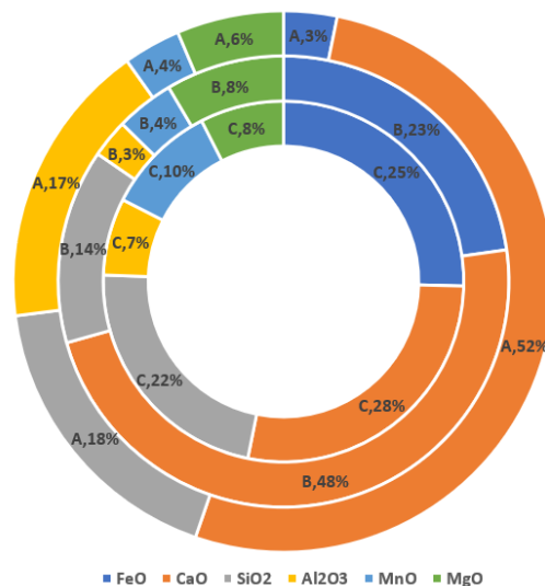
Fig. 1 Chemical compositions of steel slag from various literature. A) Ladle slag, B) BOF slag and C) EAF slag.
