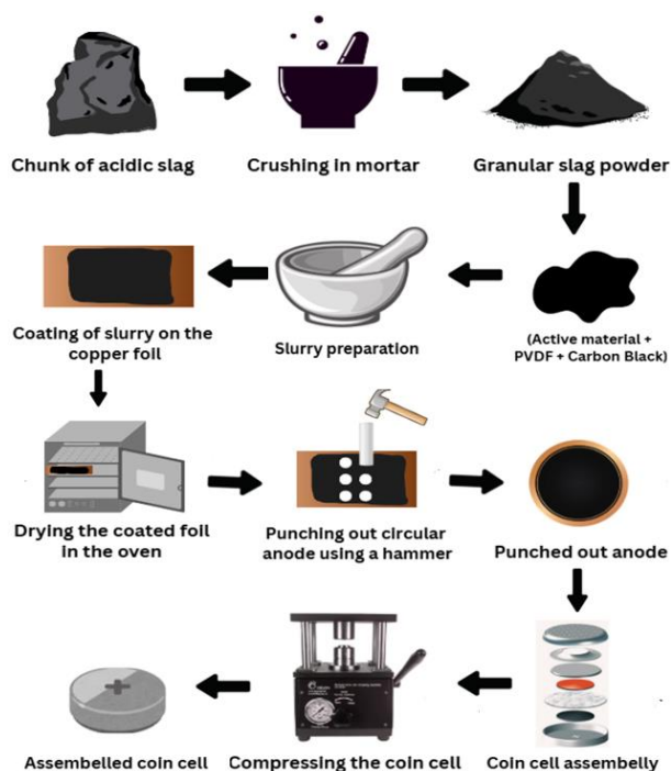
Fig. 2 Schematic of coin cell preparation from acidic steel slag.
