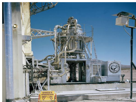
Fig. 1: Atomic reactor (Kiwi-A Prime) for studying the feasibility of nuclear rocket propulsion from Project ROVER [6].
