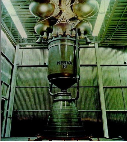
Fig. 2: NTR engine from Project NERVA [9].
