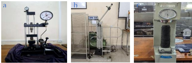
Fig. 4 (a) Universal Testing Machine (UTM), (b) Digital Impact Test Machine, (c) Brinell Hardness Testing Machine.
