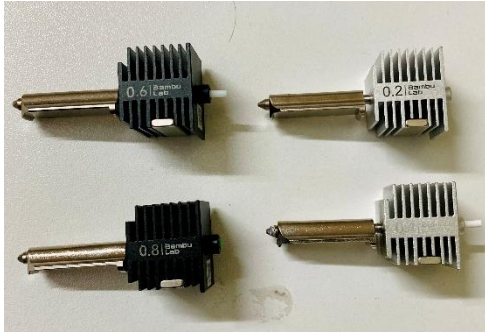
Fig. 1 Four nozzle diameters (0.2 mm, 0.4 mm, 0.6 mm, and 0.8 mm)
