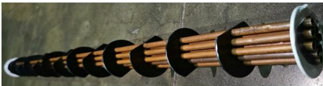
Fig.4. Photographic views of the tube bundle
