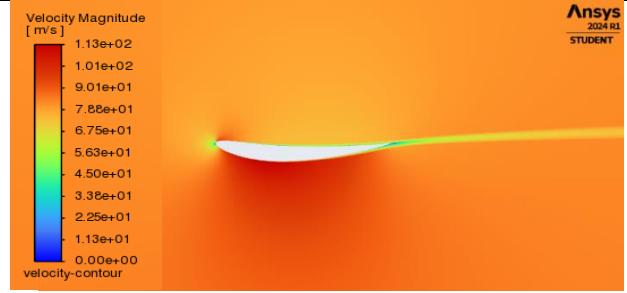
Fig. 10. NACA 6409 velocity contour
