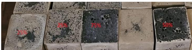
Fig. 11 Change of Color and Blow Hole on Surface of Composites Made with PFA.
