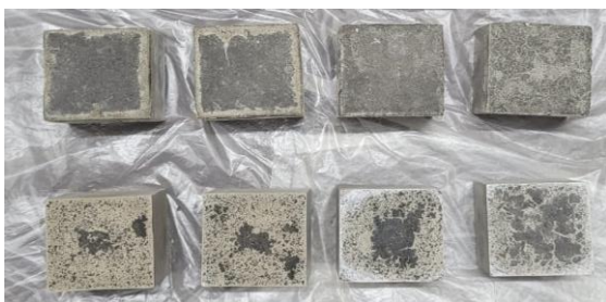
Fig.12 Changing color with increasing rate of PFA, lower row left to right for 25% PFA alkali-activator ratio-1,1.5,2,2.5. Upper row left to right for 50% PFA alkali-activator ratio-1,1.5,2,2.5.
