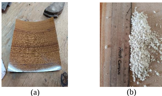
Fig.1 (a) Formica Sheet, (b) Expanded Perlite Particle
