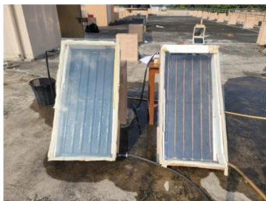
Fig.2 Experimental setup of FPC with conventional circular riser tubes (right) and rectangular riser tubes (left).
