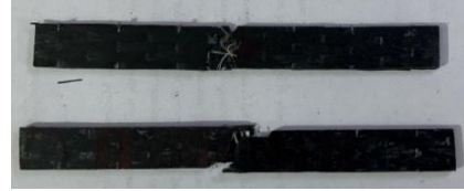
Figure 6: Schematic size Impact specimen after test
