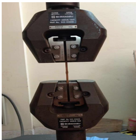
Figure 3: Tensile test on UTM (Universal Testing Machine)
