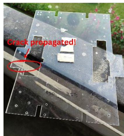
Fig.5 Crack propagation in base of assembly version 1.
