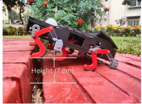
Fig.15 GiAnt ascending a 7 cm pavement.
