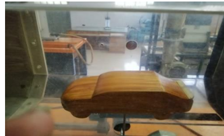
Fig 2.3.6 Experimental setup of Model Passenger Car with Rear spoiler
