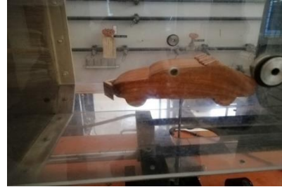
Fig 2.3.5 Experimental setup of Model Passenger Car with Delta Shape VG and V Shape Front Air Dam
