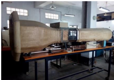
Fig 2.3.2 Wind tunnel of our laboratory
