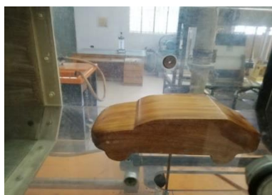
Fig 2.3.3 Experimental setup of Model Passenger Car
