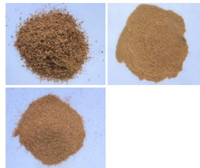
Fig.2 Raw coconut fiber after sieve analysis (particle size \geq 460 \mu\text{m} , 215-460 \mu\text{m} , 150-215 \mu\text{m} respectively)
