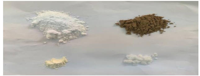
Fig.1 All components used in base mud preparation (Bentonite, Barite, Xanthan gum, NaOH respectively)
