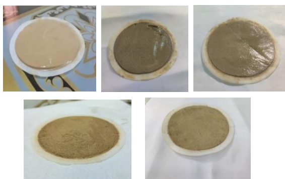
Fig.8 Mud cake formed by base fluid, sample 1, sample 2, sample 3, sample 4 respectively
