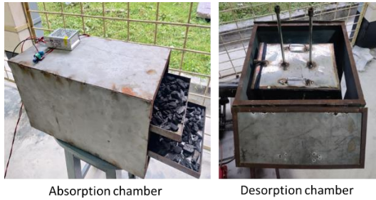
Fig. 1 Direct air carbon capture (DACC) system
