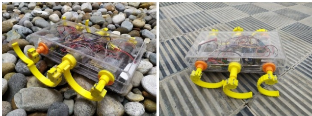
Fig. 8 Performance Test on Rough and Flat Surface
