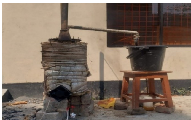
Fig. 5: Photographic view of Experimental Pyrolysis setup
