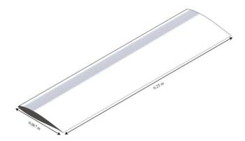
Fig.4 3D model of NACA 63-412 with different dimensions
