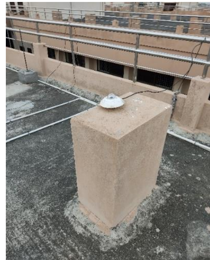
Fig.5 Measurement of global solar radiation by a pyranometer.
