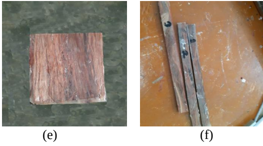
Fig. 2 (a) Laminated plate; (b) Epoxy resin and hardener mixture; (c) Fiber layer on epoxy; (d) Composite material under the heavy weight; (e) Obtained composite material; (f) Specimen cut for testing.
