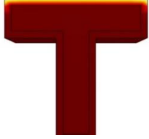
Fig.6 Heat Propagation through T-bar with Coating
