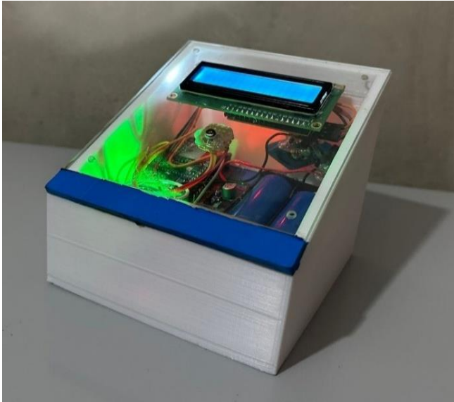
Fig. 5: Fabricated model of a phototransistor-based pyranometer
