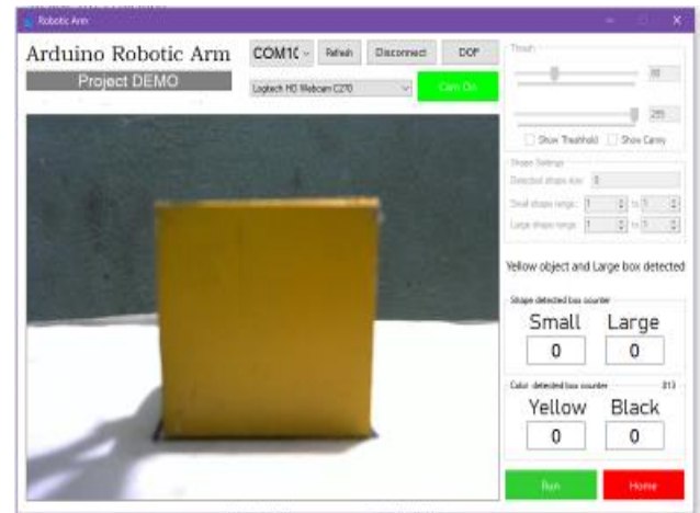
Fig. 7 OpenCV Detecting the Yellow and Large Object
