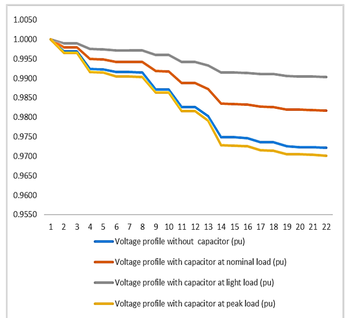
Fig. 5 The contrast of voltage profile employing SCBs at different loading conditions.
