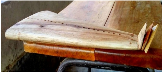
Fig. 2 Constructed wooden aircraft wing model with three winglets for the experiment in the wind tunnel
