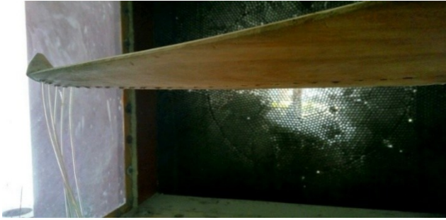
Fig. 3 The wing model placed in the test section of the wind tunnel [26] and pressure tubes are inserted to measure the static pressures
