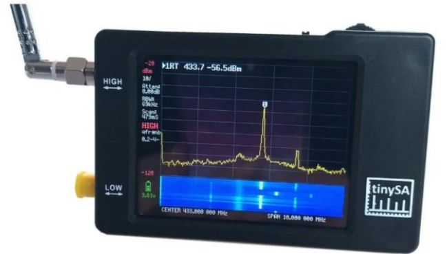
Fig. 3 TinySA spectrum analyzer used for the measurement.
