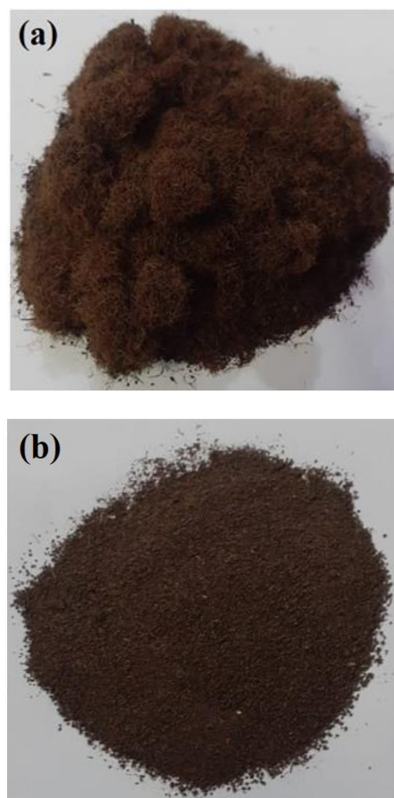
Fig. 1 Industrial tea waste powder (a) before preparation (b) after preparation
