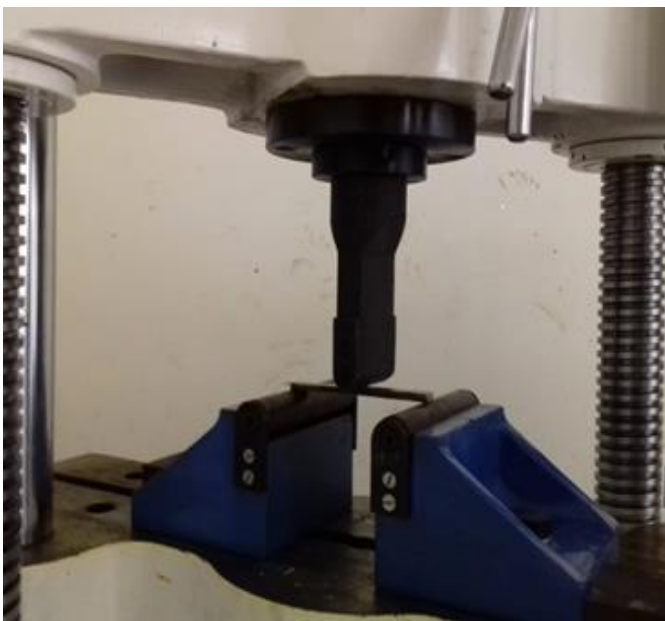
Fig. 2 Experimental setup for flexural test
