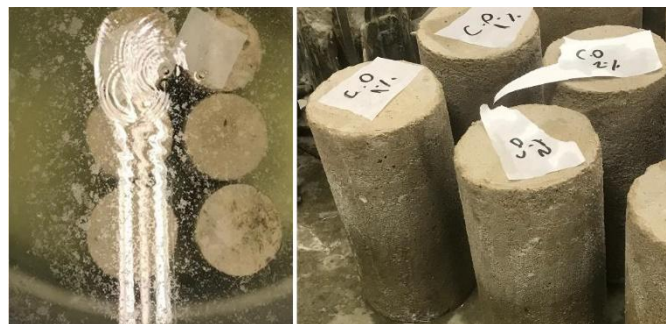
Fig. 2 The specimens were cast in molds coated with a release agent and subsequently immersed in a curing tank.
