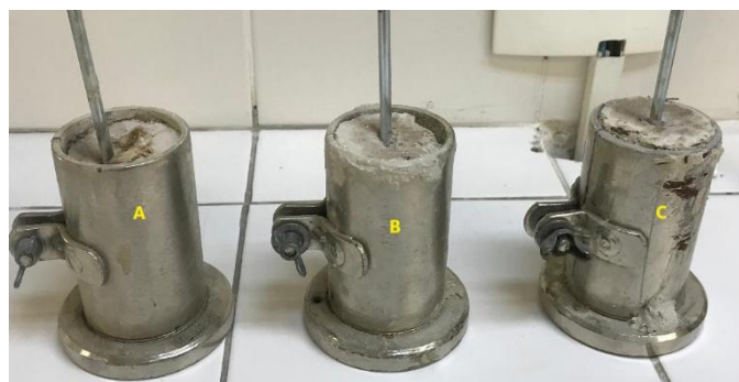
Fig. 5 Carbonation test. (A) Coconut Biomass [1% w/w]; (B) Coconut Biomass [1.5% w/w]; (C) Coconut Biomass [2% w/w].
