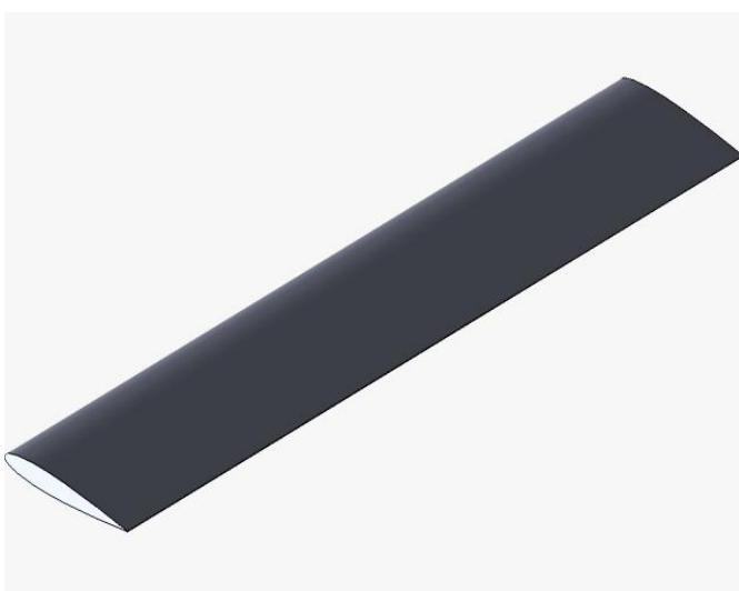
Fig. 3 3D view of NACA 0015
