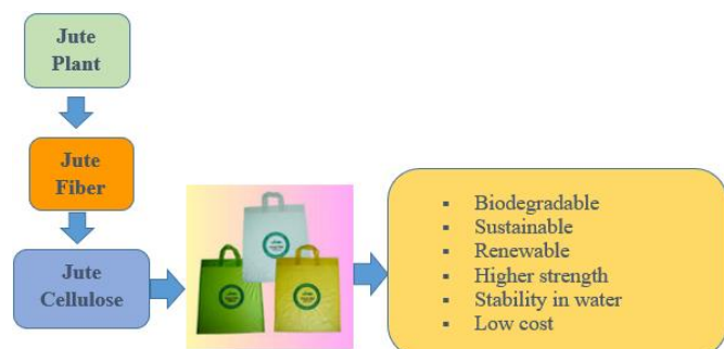
Fig. 10 Manufacturing process of eco-friendly polybags using Jute
