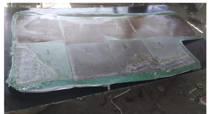
Fig. 5 Curing and demolding of composite fabricated samples
