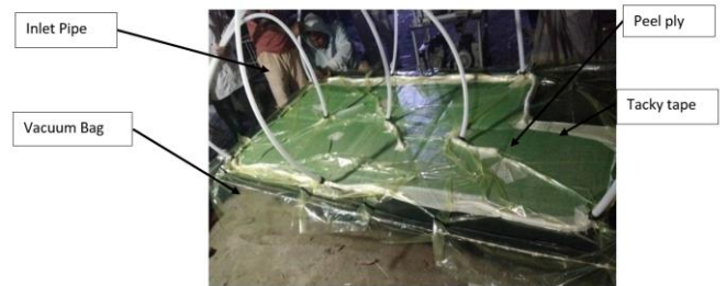
Fig. 4 Vacuum Infusion Process System Setup
