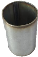
Fig. 2 Hollow stainless steel tube (Diameter = 25.4 mm and thickness = 0.4 mm)
