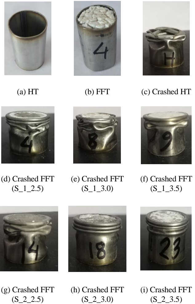
Fig. 11 (a) Hollow tube; (b) Foam filled tube; (c) Crashed hollow tube; (d) - (i) Some photographs of the crashed FFT specimens after compression tests made of S/W ratio = 1 and S/W ratio = 2 for various compaction ratios.
