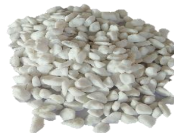
Fig. 1 Expanded perlite particles (5-6 mm)
