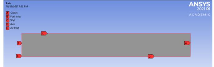
Fig. 1 2D Axisymmetric Combustor
