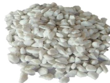
Fig. 1 Expanded perlite particles (5-6 mm)
